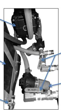
**Ball Valves for Water Supply Lines to Pump**
